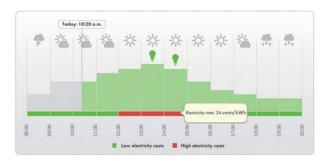
The planning screen displays the weather forecast for the plant's location and the corresponding generation forecast for the coming hours. In addition to an automatically generated timetable for the controlled appliances, the Sunny Home Manager also provides visual prompts to encourage and increase self-consumption.
