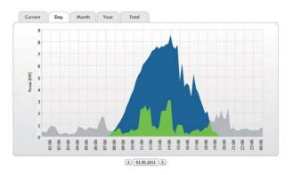
The analysis page displays the energy balance for the desired time period and facilitates a variety of generation, consumption, and self-consumption analyses.
